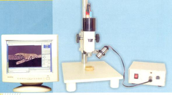
**Microscope SPM07 S** is specially designed to view & measure the weld penetration depth in welded samples by software. The test sample is mounted using cold setting resin. The surface is polished using polish papers of different grades & then with a disc polishing machine using either diamond paste or lavigated alumina powder to get scratch free mirror finish. The specimen is then etched electrolytically using an electrolytic polisher or with a chemical reagent.
